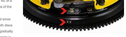
9. The adjustment feature of the floater plate is highly critical to the correct function of the clutch. If you wish to check the adjustment, see the Adjustments section (page 4) for more information.
